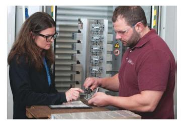
In front of the loading station of the shop's Fastems FMS One flexible manufacturing system, Angela Olsen and Mach Machine President Dan Olsen check the dimensions of lens-mount components.
